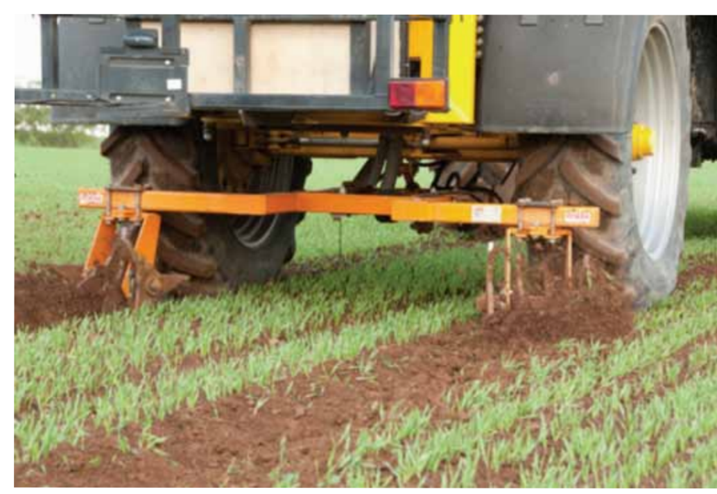
Spiked harrow unit installed on a sprayer to remove compaction following wheeling
