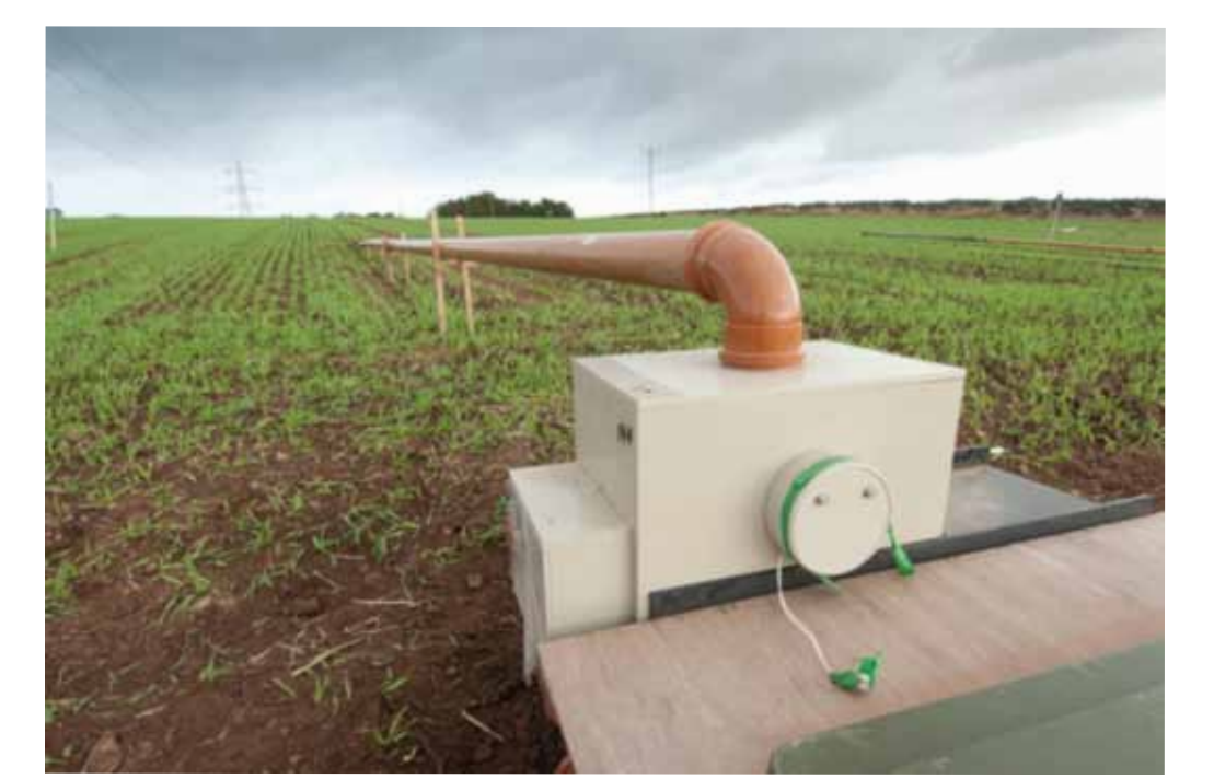
Field instrumentation to measure runoff and also collect water for chemical analysis
